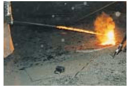
Molten metal at 1565°C poured on to a multi-conductor VIBRAFLAME® cable under tension.
